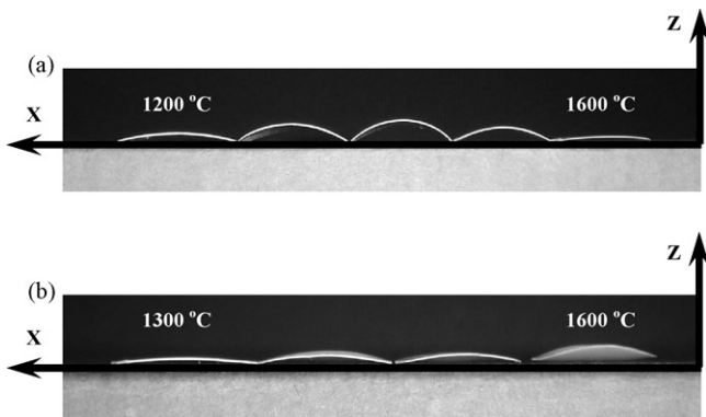
Fig. 5. Distortion characteristic of the round-shape specimen ( x - z plane view) at various temperature. (a) sintering deformation of Type-I structure specimen; (b) sintering deformation of Type-II structure specimen.
